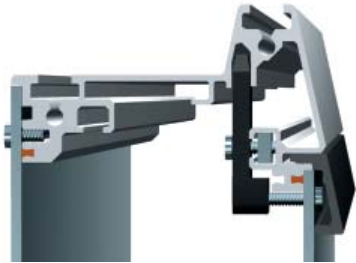
Front panel installation screwed from front
