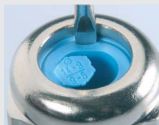
Fig. 3 With a large cable diameter – remove inlet. Insert screwdriver vertically into separating seam
