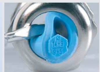
Fig. 4 Lift out the inlet
